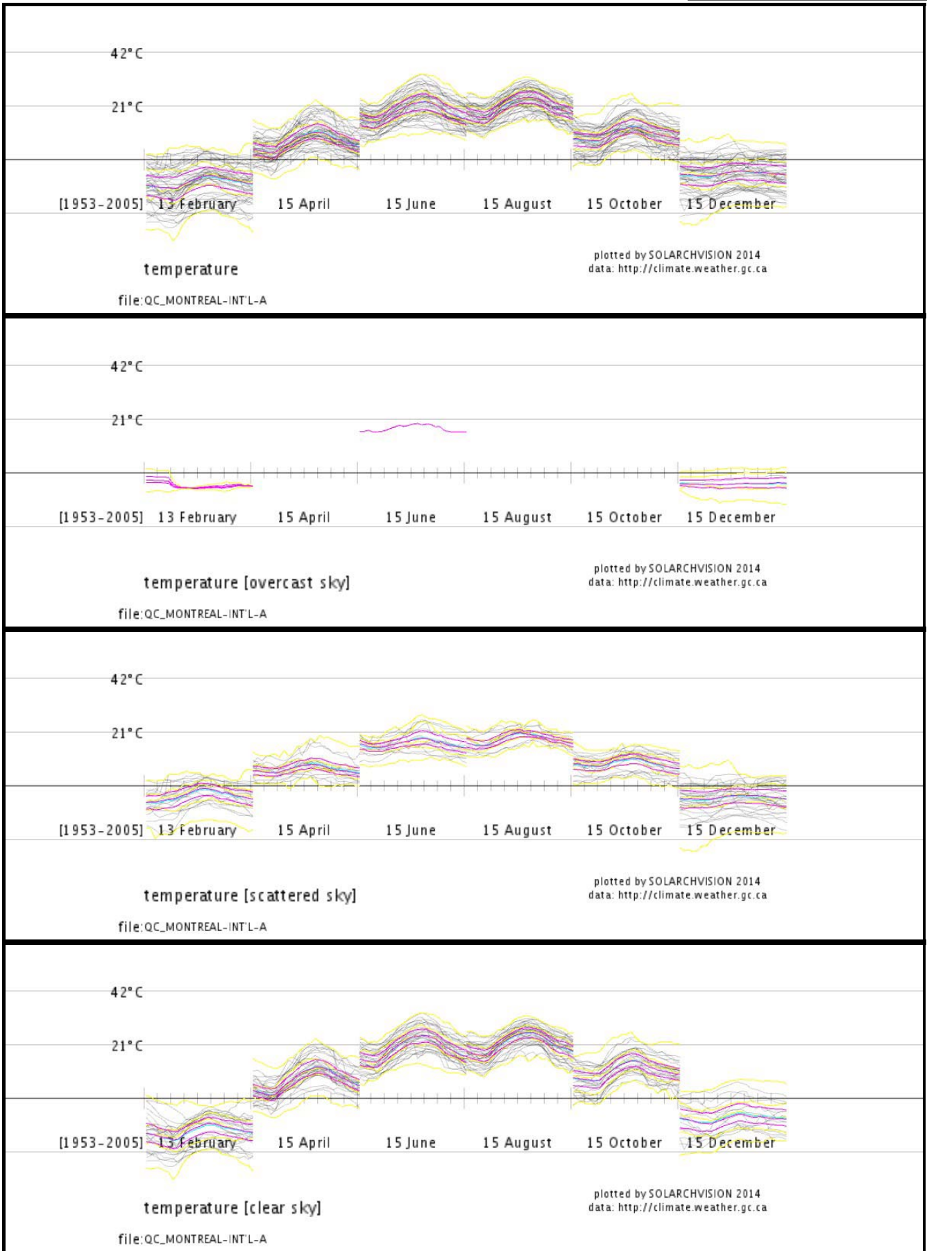
Fig. B1-B4: 1953-2005 hourly temperature models in different months with the mean, average high, average low, max. and min. values in general and different sky conditions (clear, scattered, overcast) based on CWEED files
