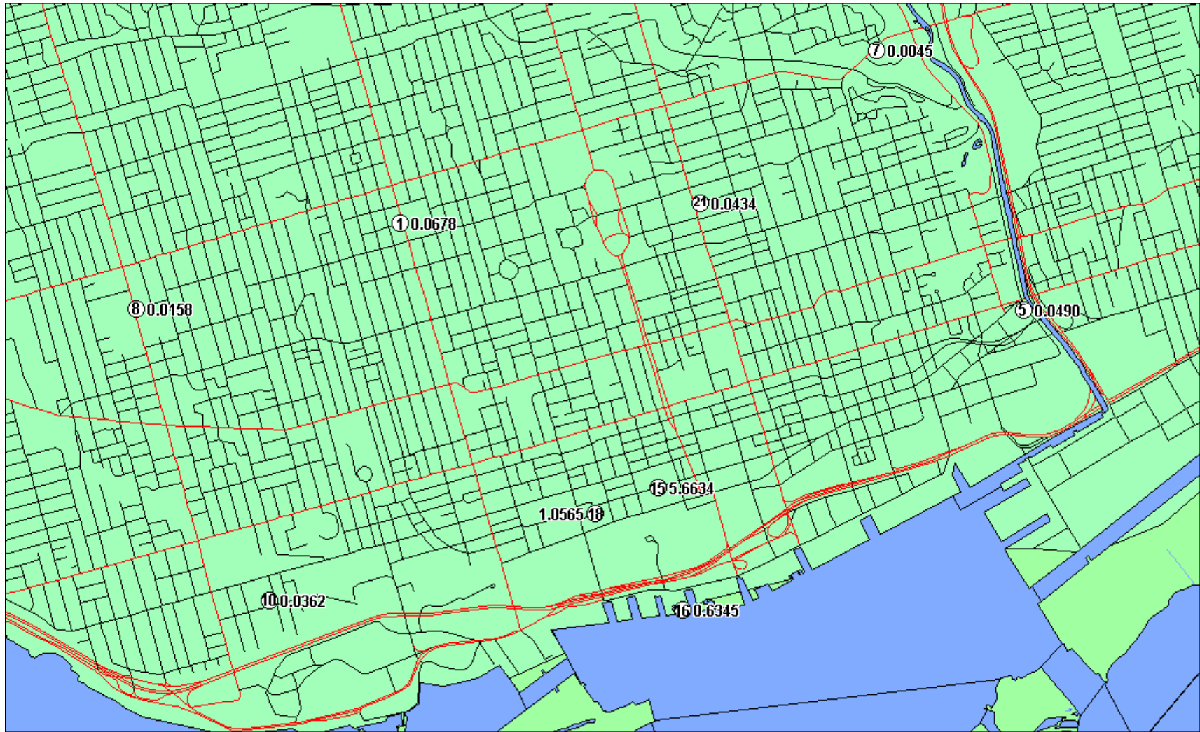
Figure No. 05 Normalized SC 6 Levels Recorded Based on the Maximum Received Signal in Downtown Toronto (Percent of Limit)
