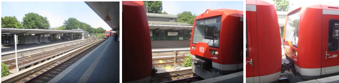
Hamburg S-Bahn docking of S1 train from Poppenbüttel onto a train from the Airport
