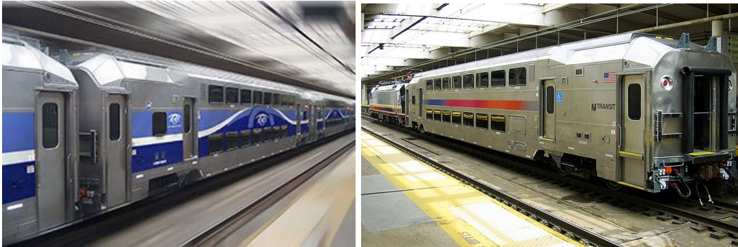
Left: AMT Bombardier multilevel car with high & low floor doors right: NJTransit Bombardier multilevel car with high & high/loor floor doors
